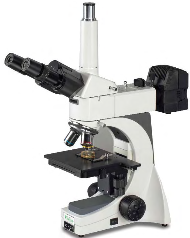
The pre-focus prevents objectives colliding with the specimen.
